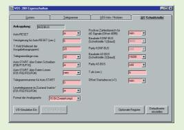
As part of the commissioning process, the WINCONF program is used to setup and configure the automation system interface parameters and the I/O units. This information is created off-line using easy to follow menus and stored to disk for downloading to a nonvolatile memory within the VOS 200.
