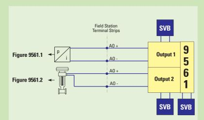
The Type 9561 is designed to provide intrinsically safe connections to two control valves, i/p transducers or displays located in Zone 0,1 gas group IIC or a Class I, Division 1 or 2 hazardous area. The two outputs are mutually independent, short-circuit-proof and galvanically isolated.
