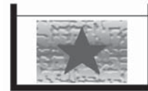
Ex-m encloses all ignitable component parts in resin, preventing contact with explosive gases.
