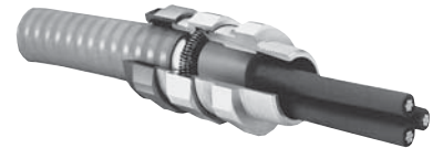
TMCX Terminator™ cable fittings for use with Type MC-HL or ITC-HL cable in Class I, Division 1 locations.
