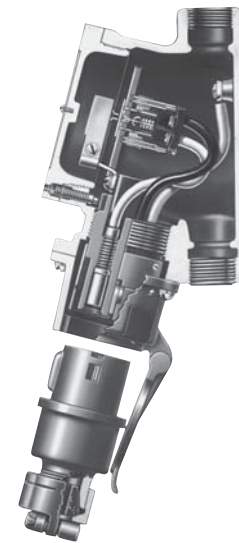
Receptacle constructed with an interlocked switch. Rotating the plug after insertion actuates this switch. This is also referred to as “dead front.”
