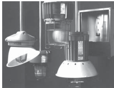
Crouse-Hinds luminaires are certified as ExnR "restricted breathing" for Division 2 locations
