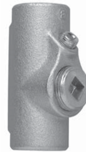
EYSX Series – For sealing in vertical or horizontal conduit runs. Class I, Groups A, B, C, D, and Class II, Groups E, F, and G.
