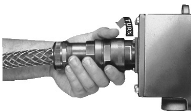
C. Turn plug clamping nut an additional 45° counterclockwise to the release position, thereby effecting delayed action.
